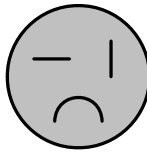
Figure 4-10. Tandem Prong-type Plug
