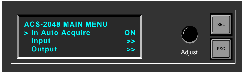
Figure 2-2. Display Section with Main Menu
