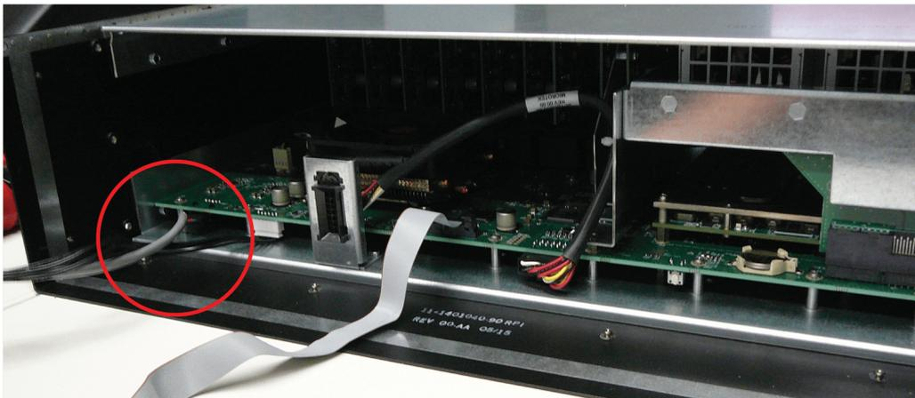
Image 15-35 USB Ext Cable connected to the Motherboard
